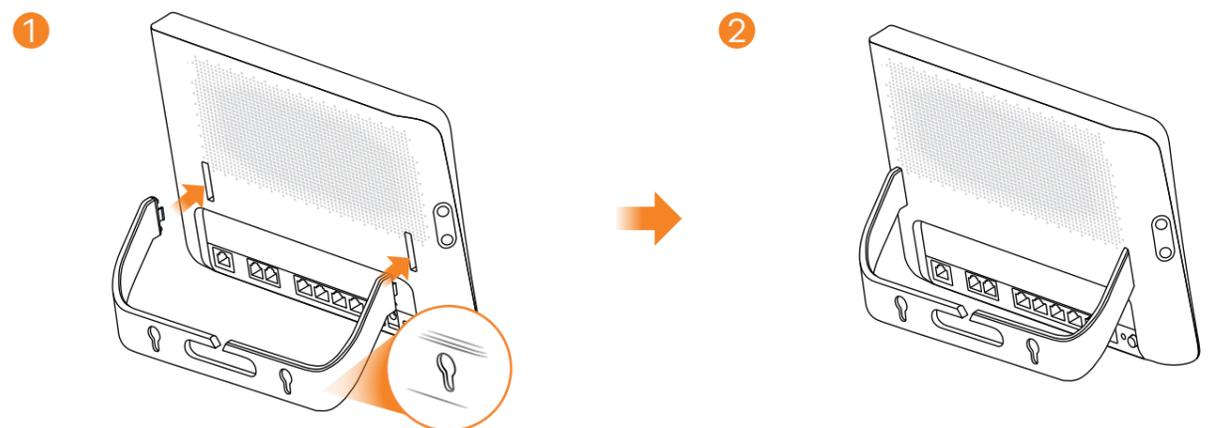
**EN** Drill two holes at the distance of 115mm apart. Insert screw anchors and screws (not provided) into the holes. Attach the bracket to your VMG8823-BX0B with the bracket holes facing down. Hang it on the screws.
