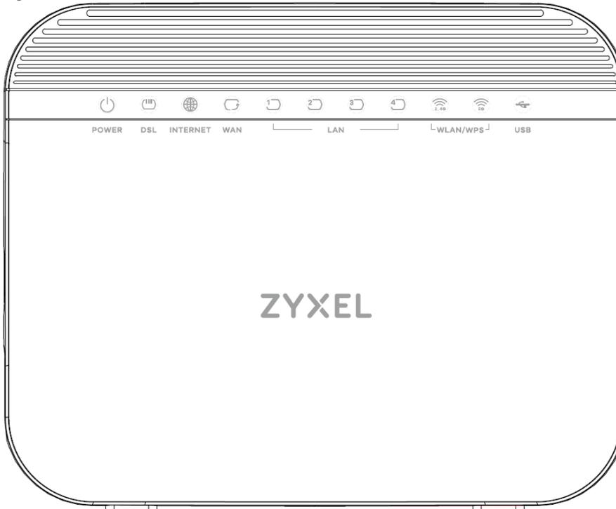
Figure 13 VMG3625-T50A Front Panel
